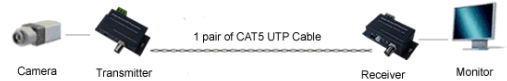
Active CAT5 Video Transceiver over 3000ft CAT5 Cable Video Transmission in CCTV system
