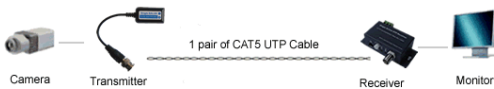
Passive & Active CAT5 Video Transceiver over 3000ft CAT5 Cable Video Transmission in CCTV system
